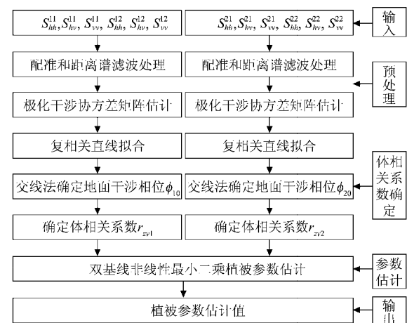
图8 双基线极化干涉三层植被参数反演流程图 Fig.8 Low chart of parameters inversion of the three-layer vegetation by double-baseline Pol-InSAR
